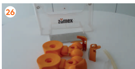
26 Once we have all the pieces disassembled, we proceed to clean them with a degreasing disinfectant.
