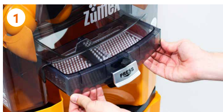
1 Remove the juice container and the cover .
