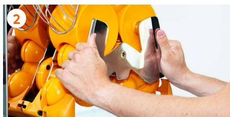
2 Remove 1Step Extraction kit and the blade .
