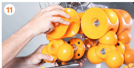
11 Unscrew the securing knobs of the pressing units. Take off the pressing units in pairs.
