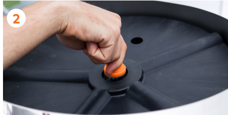
2 Take off the feeder plate by unscrewing the central knob.
