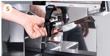
5 Remove the Speed Up Tap by easily unscrewing it.
